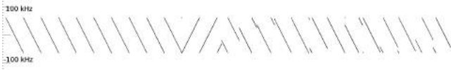
Figure 12.8: The Authors' Recording [58] of a DL Transmission by a LoRa Gateway Node towards Arduino (Atmel AVR) Node [3] Equipped with a LoRa Shield [2] Presented in Inspectrum [72]
