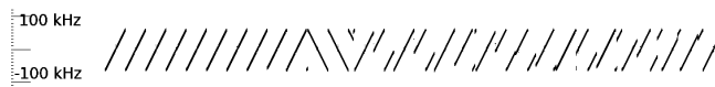
Figure 12.7: The Authors’ Recording [58] of an UL Transmission by an Arduino (Atmel AVR) Node [3] Equipped with a LoRa Shield [2] Presented in Inspectrum [72]
